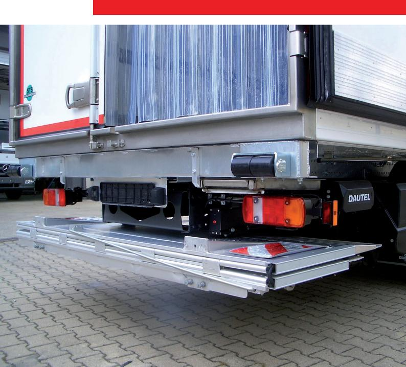
DAUTEL *SLIDER* DS 1500/2000VA has proven itself for years in tough daily use in shipping companies and transport operations. With a powerful load torque of 15/20 kNm or a rated load of 1500/2000 kg at a load centre of 1000 mm, measured at the centre from the beginning of the platform, these are the first choice when working with heavy loads.
