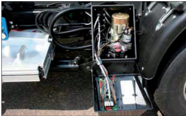
Service-friendly drive unit and control unit
