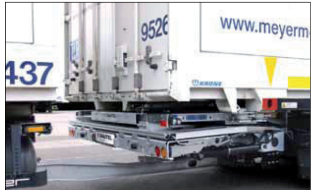
DS 1500/2000VT XXL for BDF high-volume freight transport C 782, HGV driving height of 860 mm
